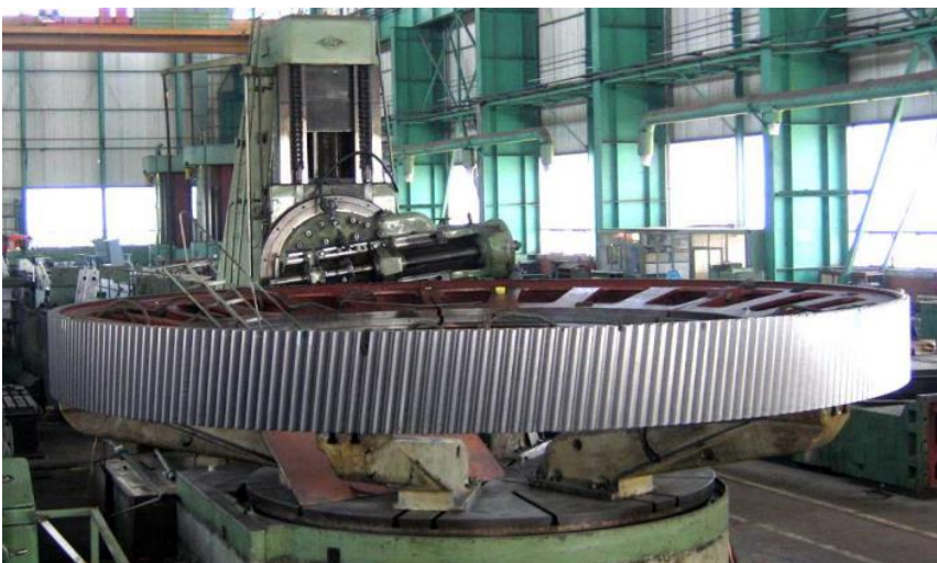
Driven gear, 6700mm diameter
