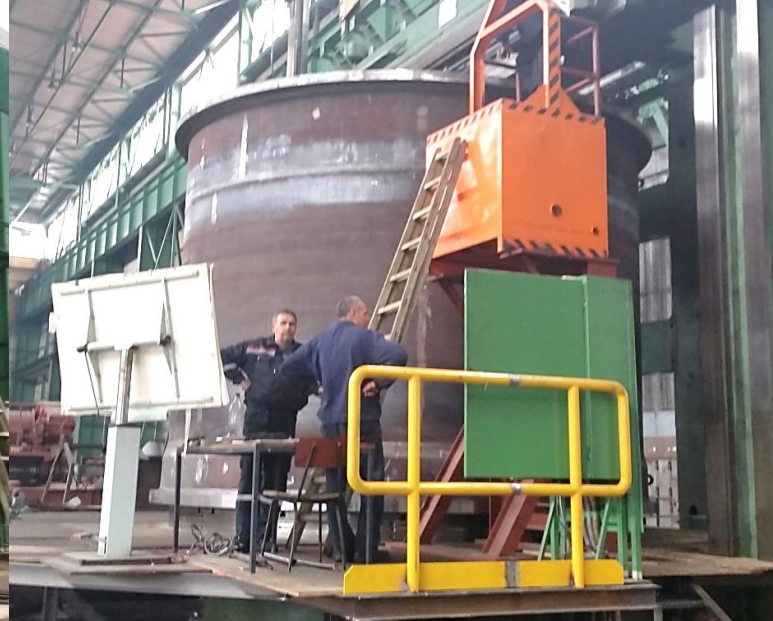
Mill Shell, RTB Bor Serbia, 5500x8500mm
